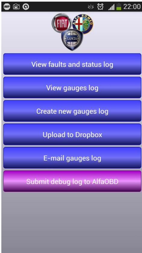
“View faults and status log” behaves differently depending on the initial screen from which Tools screen is opened. If Tools screen is open from the first AlfaOBD screen, a push on the “View faults and status log” displays a list of all available logs recorded earlier. Select a log to view, the log will be opened with a text editor. If Tools screen is open from the AlfaOBD second screen, a push on the “View faults and status log” displays the log for the selected or connected ECU.
