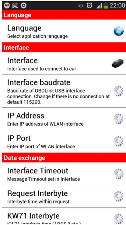
The OBD interface used is selected in the "Interface" list. AlfaOBD verifies the type of the interface connected during connection to a car ECU. If a wrong interface selected in the preferences, AlfaOBD can correct the selection.
