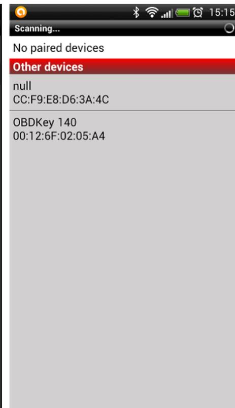
Complete pairing with the interface and select it in the list, AlfaOBD will return to the first screen and automatically set connection to the selected interface.
