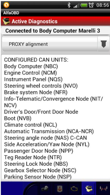
For most of the procedures it is important that engine is NOT running (but the key is in MAR), this is expected by default. For the procedures for which it is essential that the engine IS running, it is specifically noted in the on-screen guidance. Follow the on-screen instructions to perform procedures. For some of the procedures certain conditions, additional checks, steps, or data entry are necessary, just follow the guidance.
